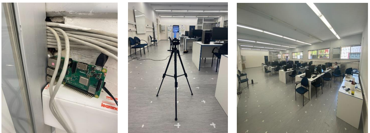
Figure 4-7: Testbed setup: Raspberry Pi AP (left); tripod (center); indoor area/lab 206 (right).
