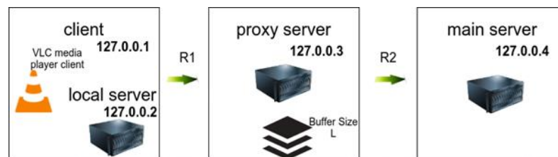
Figure 3-2: Implementation with an intermediate cache server
